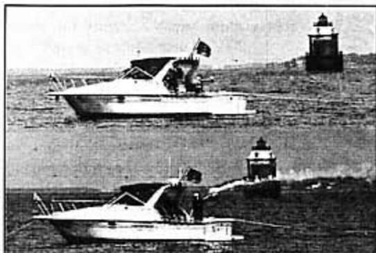
All hand-held flares have limited use in daylight conditions but SOLAS flares (bottom) offer significantly more brilliance and secondary smoke.
